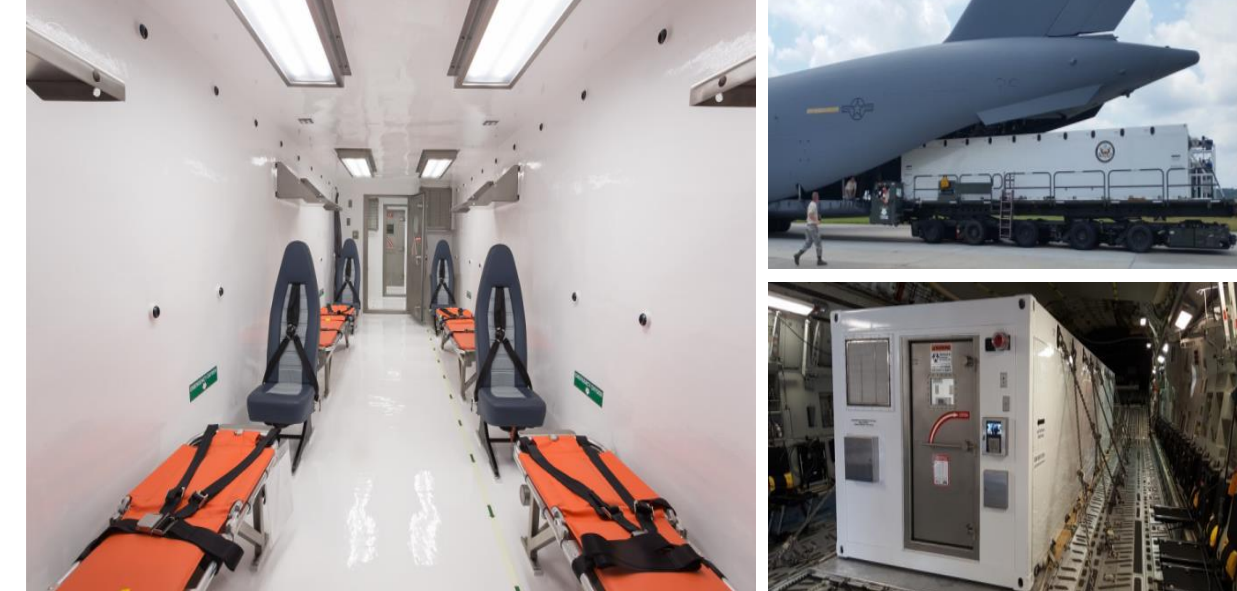
Patient transport container for safe evacuation of people infected with highly contagious diseases (e.g., Ebola)
