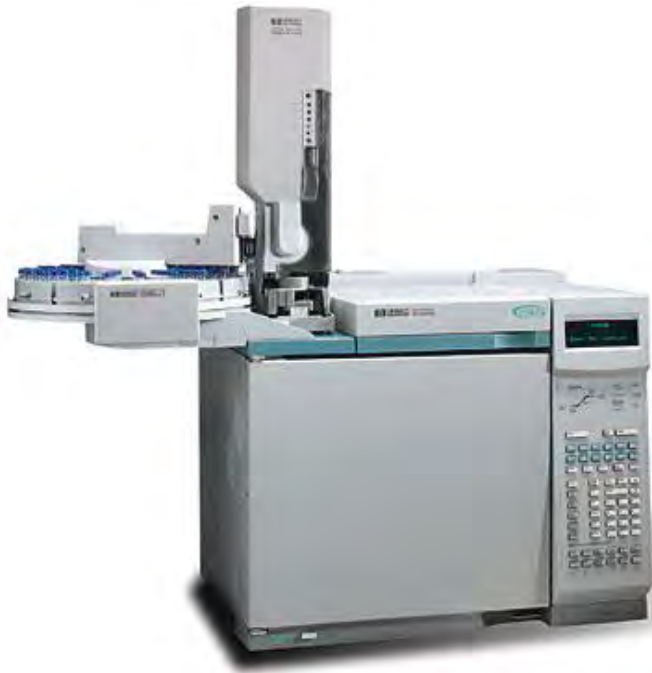
Agilent GC + Gerstel System used to interface to and test performer identification modules
