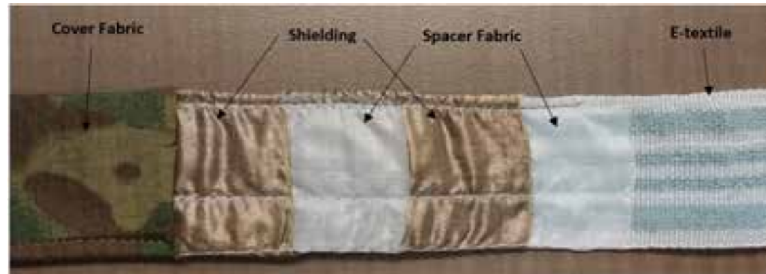
Cutaway of E-textile power and data network showing double layer of EMI shielding.
