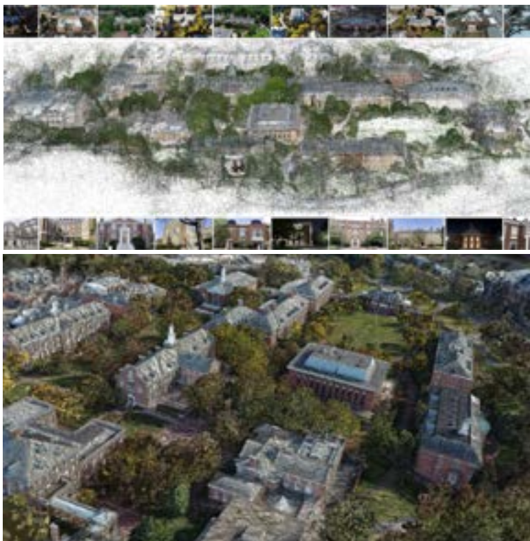
Example 3D site models created of the Johns Hopkins University Campus using WRIVA technologies. These examples were created using still images collected at a variety of lighting and environmental conditions and from different camera and altitudes
